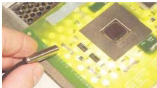
*Figure 2. Flexible endoscope under a tape ball grid array.*
