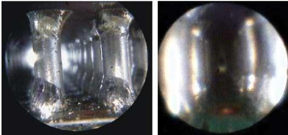
Figure 3 (left). This image shows a row of columns under a CCGA. Figure 4 (right). This image shows the central area under a CCGA.
