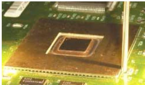
*Figure 1. Rigid endoscope shown adjacent to a tape ball grid array.*
